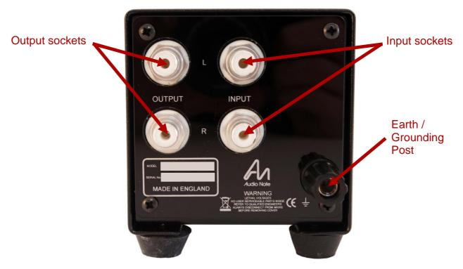
Once located, connect the AN-S4 between your turntable and phonostage input. Connect your tonearm / turntable output cables to the input sockets on the AN-S4, and the output sockets of the AN-S4 to your MM phonostage input. It is important to use good quality, shielded interconnects for all turntable connections; this will help to minimize any noise or hum problems.
